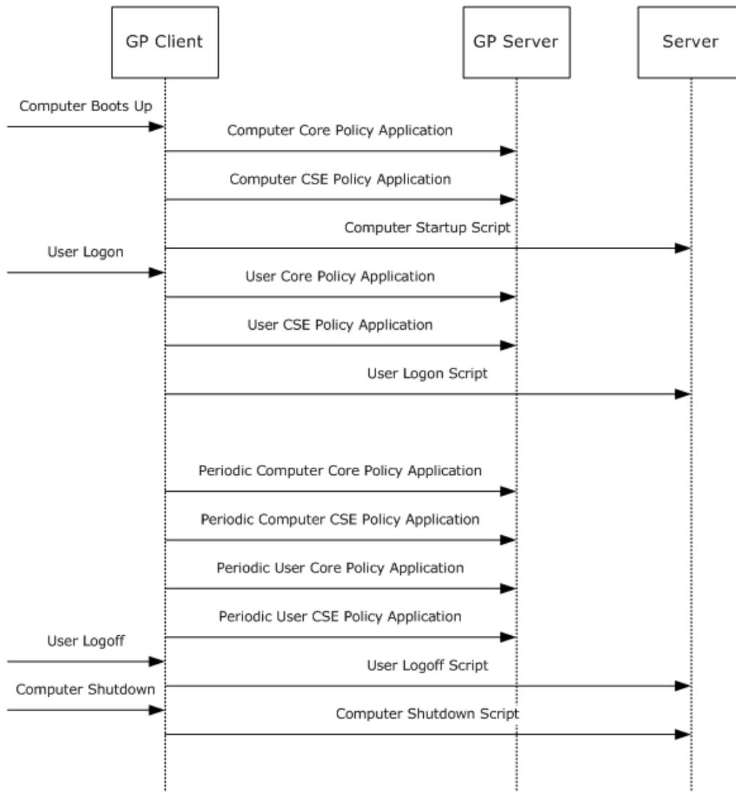
**Figure 7: Group Policy System Processing internal architecture**
