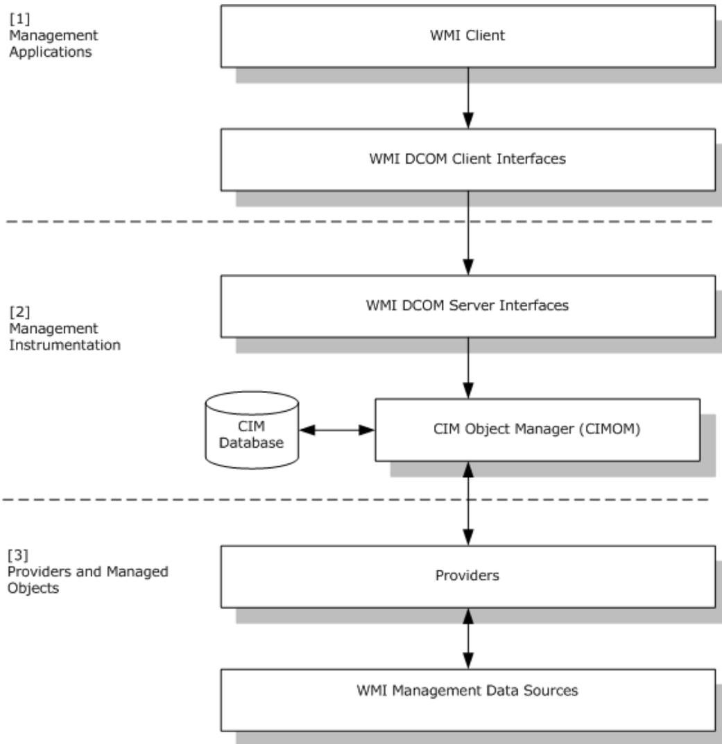
**Figure 1: Windows Management Instrumentation Remote Protocol architecture**
