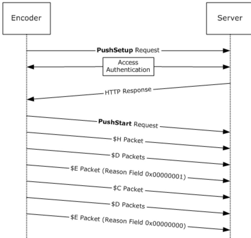
**Figure 4: General push distribution sequence with \$C packet**
