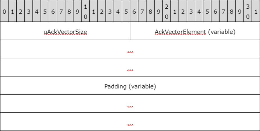
**AckVectorElement (variable):** An array of ACK Vector elements. Each element is composed of a state, and the number of contiguous datagrams that share the same state.
