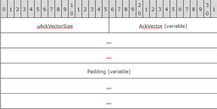
**AckVector (variable):** A variable size array of ACK Vector Elements (section 2.2.2.7.1). The size of the AckVector field is specified by the uAckVectorSize field.
