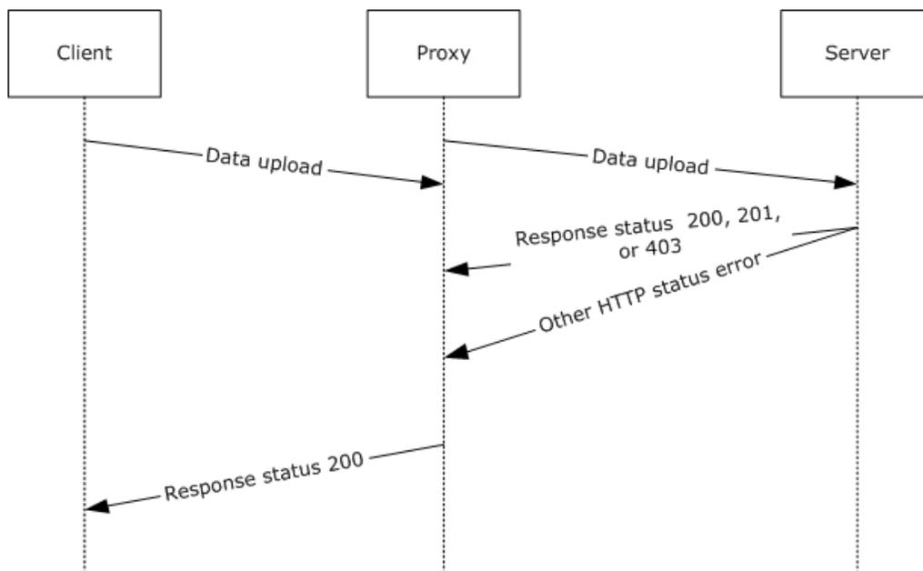
**Figure 11: Client upload through a proxy server**
