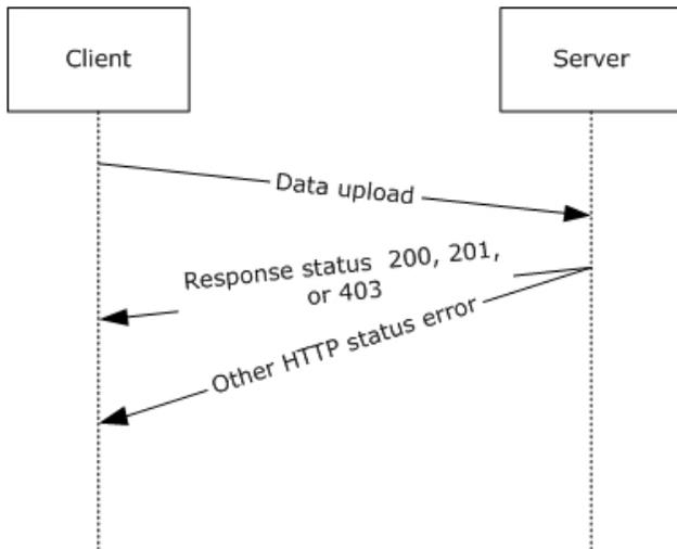
**Figure 9: Client-to-Service data upload and response**
