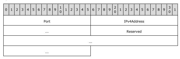
**Port (2 bytes):** This field MUST NOT be used and MUST be reserved. The server SHOULD set this field to zero, and the client MUST ignore it on receipt.
