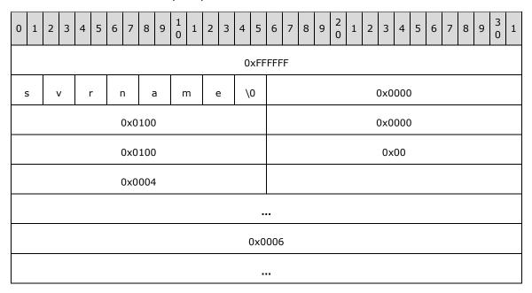
The example response package's **IPv4\_DNS\_ADDRESS** field contains four elements of the **SOCKADDR\_STORAGE** structure, and the **IPv6\_DNS\_ADDRESS** field contains six elements of **SOCKADDR\_STORAGE** structure.
