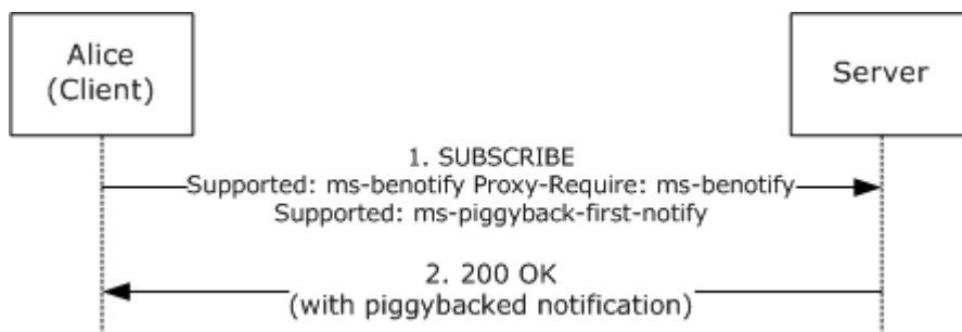
Figure 3: Batched SUBSCRIBE request and piggybacked NOTIFY example
