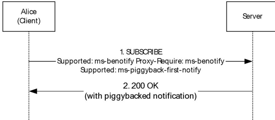
**Figure 3: Batched SUBSCRIBE request and piggybacked NOTIFY example**
