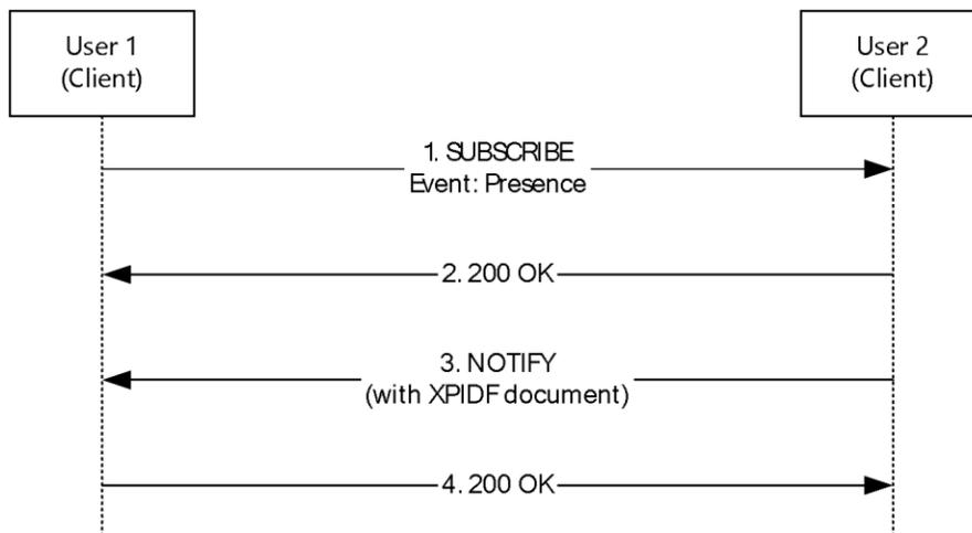
**Figure 11: P2P subscription and XPIDF presence format example**
