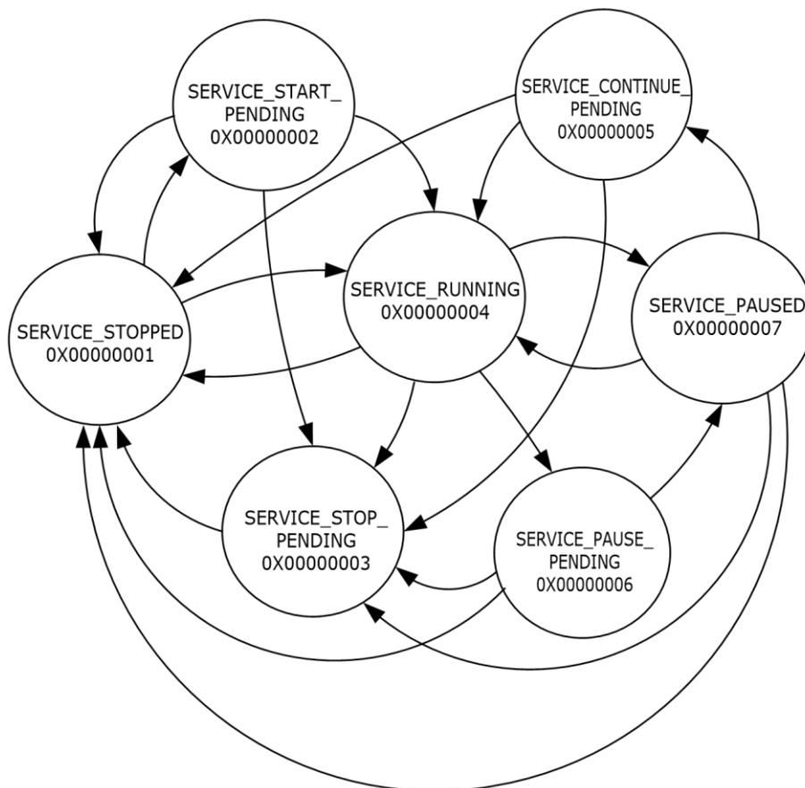
**Figure 1: State Diagram in which life cycle and execution properties are governed by the rules defined in SCM**
