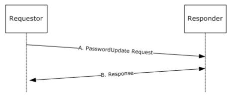
Figure 1: A requestor makes a PasswordUpdate request
