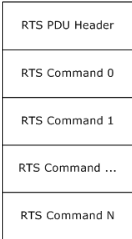
Figure 12: RTS PDU structure
