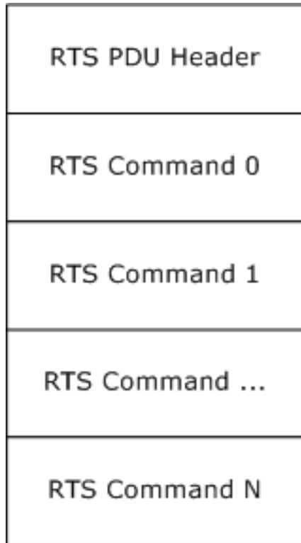
Figure 12: RTS PDU structure
