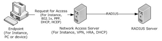
Figure 1: Common RADIUS deployment model
