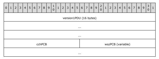
**version1PDU (16 bytes):** The RDP\_PRECONNECTION\_PDU\_V1 header, as specified in section 2.2.1.1.
