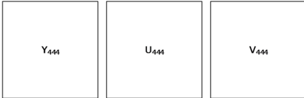
Figure 6: A representation of a YUV444 frame as three planes
