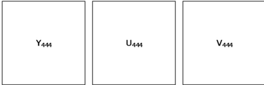
Figure 8: A representation of a YUV444 frame as three planes
