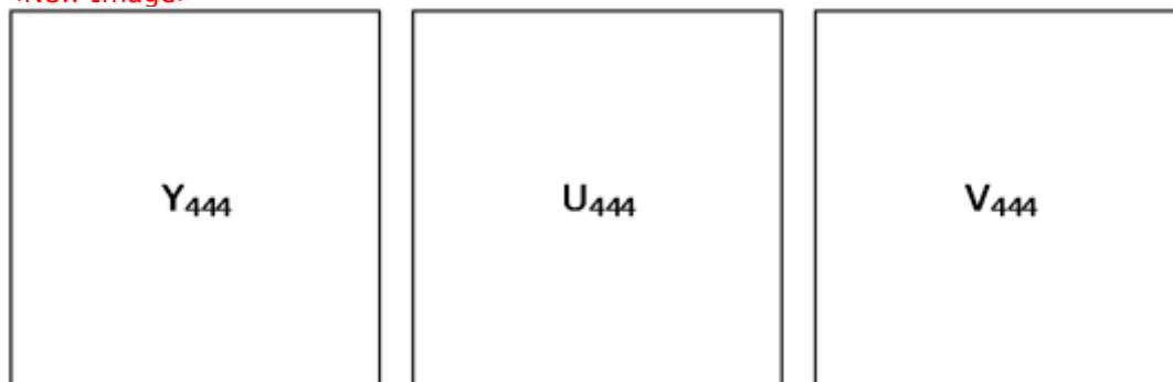
Figure 8: A representation of a YUV444 frame as three planes
