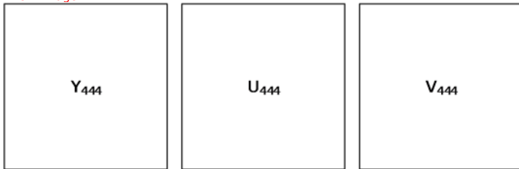
Figure 6: A representation of a YUV444 frame as three planes
