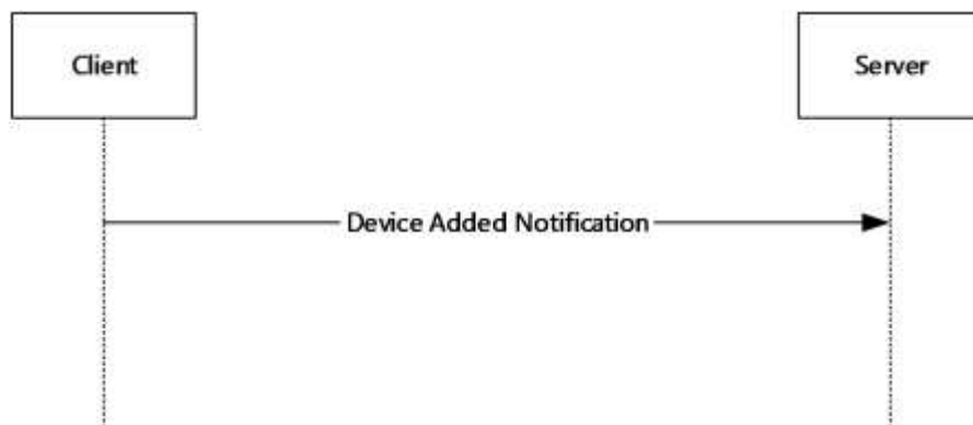
Figure 2: New Device sequence
