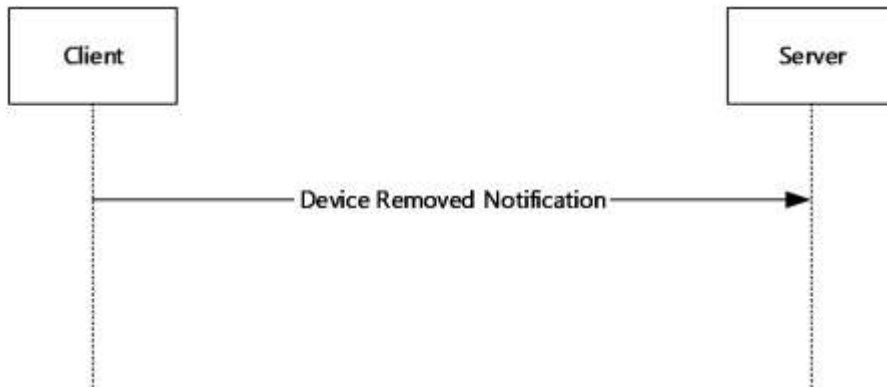
Figure 3: Device Removal sequence
