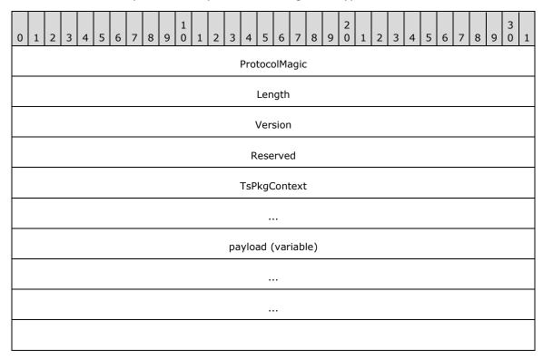
ProtocolMagic (4 bytes): A 32-bit integer that MUST be equal to the value 0x4eacc3c8.
