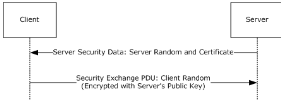
Figure 9: Client and server random value exchange
