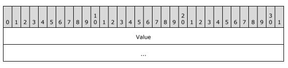
**Value (8 bytes):** This field specifies an unsigned integer representing a timestamp value in network byte order. The unit of measurement MUST be in 100 nanosecond units.
