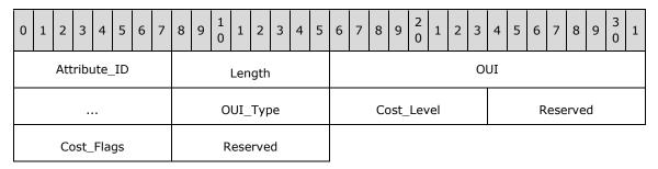
**Attribute\_ID (1 byte):** Contains the ID of the element as specified [IEEE802.11-2007] section 7.3.2. It MUST contain a value of 221 (OxDD), identifying a vendor-specific element (as specified in [IEEE802.11-2007] table 26) in which the vendor is identified by an IEEE-issued OUI.
