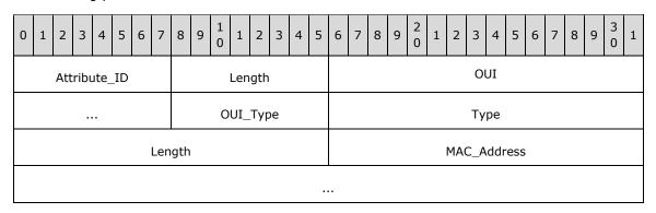
**Attribute\_ID (1 byte):** Contains the ID of the element as specified [IEEE802.11-2007] section 7.3.2. It MUST contain a value of 221 (0xDD), identifying a vendor-specific element (as specified in [IEEE802.11-2007] table 26) in which the vendor is identified by an IEEE-issued OUI.
