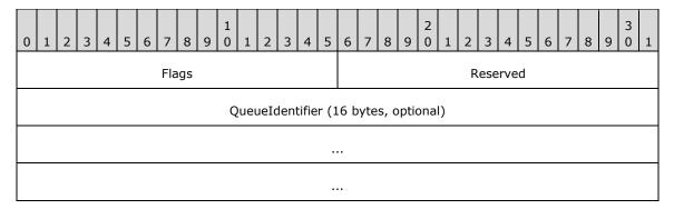
**Flags (2 bytes):** A 16-bit unsigned short integer field that provides bit flags containing additional information about the packet.
