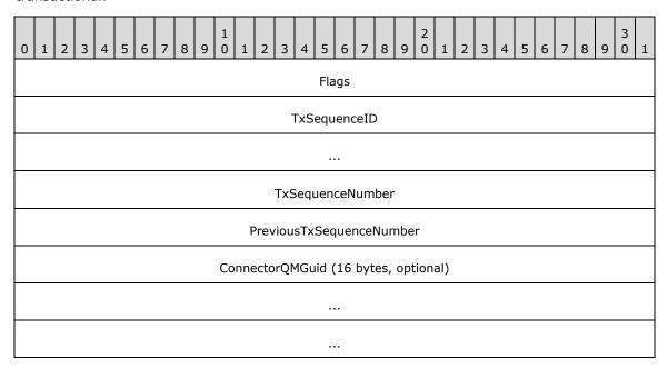
**Flags (4 bytes):** A 32-bit unsigned integer that contains a set of options that provide additional information about the packet. Any combination of these values is acceptable unless otherwise noted in the following table.
