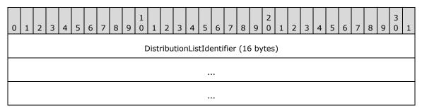
**DistributionListIdentifier (16 bytes):** A **GUID**, as specified in [MS-DTYP] section 2.3.4, that MUST identify a **distribution list**. The start of this field is rounded up to the next 4-byte boundary.
