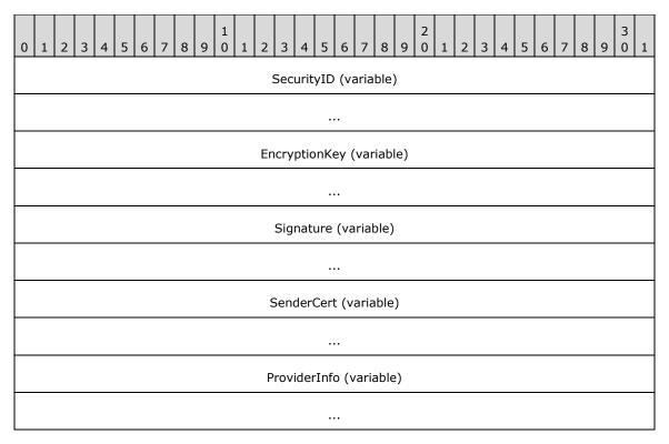
**SecurityID (variable):** Contains the sender SID or the sending queue manager GUID. This field MUST be set to the queue manager **GUID** when the packet is sent and signed by the queue manager.
