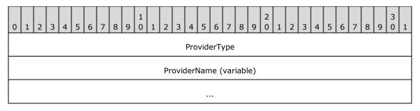
**ProviderType (4 bytes):** A 32-bit unsigned integer that indicates the type of the alternative provider used to produce the signature.
