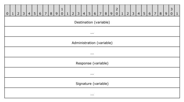
**Destination (variable):** An MQFAddressHeader that specifies the name of one or more destination queues. This field MUST contain the list of all queues that were sent a copy of this UserMessage Packet. The end of this field is rounded up to the next 4-byte boundary. There are no restrictions on the value of the padding bytes.<a href="tel:40"><10></a>
