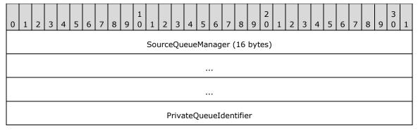
**SourceQueueManager (16 bytes):** A **GUID**, as specified in [MS-DTYP] section 2.3.4, that MUST specify the queue manager that hosts the private queue. The start of this field is rounded up to the next 4-byte boundary.
