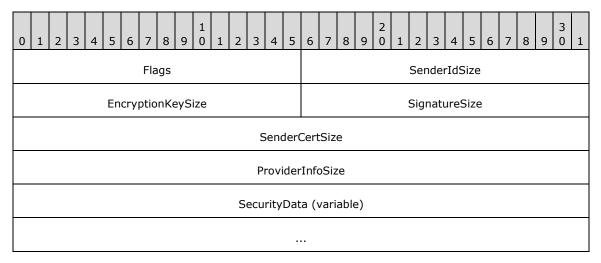
**Flags (2 bytes):** A 16-bit unsigned short integer that contains a set of options that provides additional information about the packet. Any combination of these values is acceptable unless otherwise noted in the following table.
