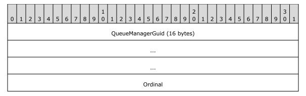
**QueueManagerGuid (16 bytes):** A **GUID**, as specified in [MS-DTYP] section 2.3.4, that contains the identifier of the sender queue manager. This value MUST be the same for messages originating from the same queue manager.
