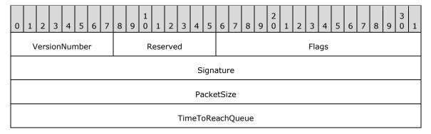
**VersionNumber (1 byte):** An 8-bit unsigned integer that is the version of the packet format. This field MUST be set to the value 0x10.
