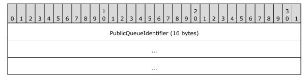
**PublicQueueIdentifier (16 bytes):** A **GUID**, as specified in [MS-DTYP] section 2.3.4, that MUST be set to the identifier of the public queue.
