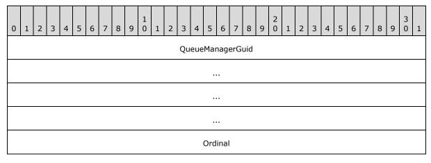
**QueueManagerGuid (16 bytes):** A **GUID**, as specified in [MS-DTYP] section 2.3.4, that contains the identifier of the sender queue manager. This value MUST be the same for messages originating from the same queue manager.
