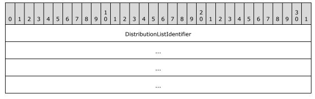
**DistributionListIdentifier (16 bytes):** A **GUID**, as specified in [MS-DTYP] section 2.3.4, that MUST identify a distribution list. The start of this field is rounded up to the next 4-byte boundary.
