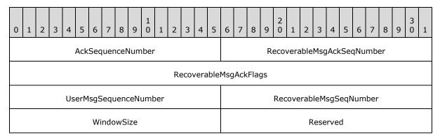
**AckSequenceNumber (2 bytes):** A 16-bit unsigned integer that specifies a count of messages received. This field MUST be set to the count of UserMessage Packets received on this session. This field acknowledges all messages up to and including the specified sequence number. This field has a valid range from 0x0000 to 0xFFFF, inclusive.
