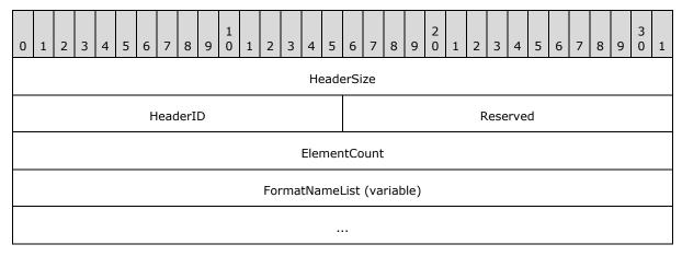
**HeaderSize (4 bytes):** A 32-bit unsigned integer that specifies the size of the header. This value MUST contain the size, in bytes, of this header including the variable data. This field has a valid range between 0x000000C and the size limit imposed by the value of **BaseHeader.PacketSize**.
