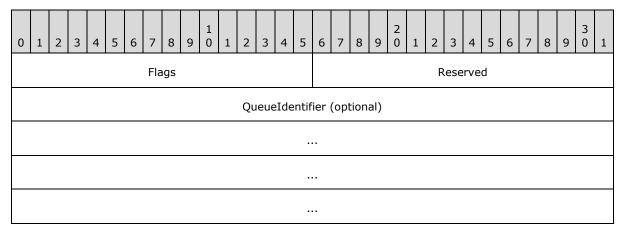
**Flags (2 bytes):** A 16-bit unsigned short integer field that provides bit flags containing additional information about the packet.
