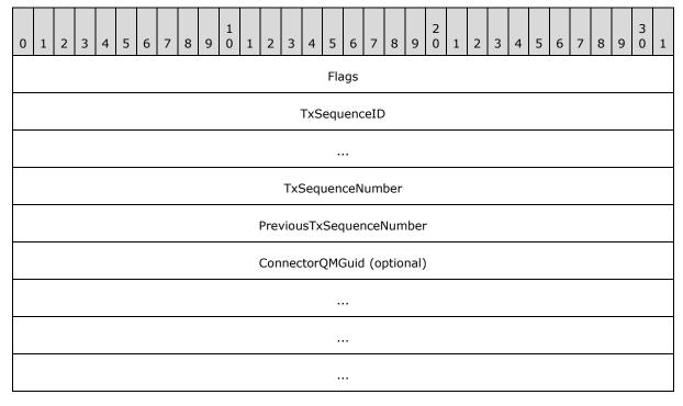
**Flags (4 bytes):** A 32-bit unsigned integer that contains a set of options that provide additional information about the packet. Any combination of these values is acceptable unless otherwise noted in the following table.
