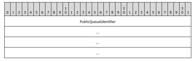
**PublicQueueIdentifier (16 bytes):** A **GUID**, as specified in [MS-DTYP] section 2.3.4, that MUST be set to the identifier of the public queue.
