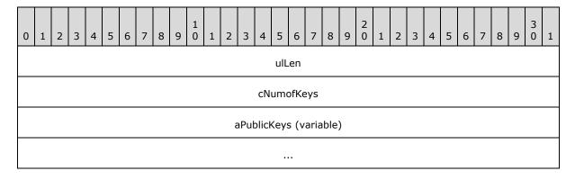
**ulLen (4 bytes):** An unsigned 32-bit integer that MUST contain the size, in bytes, of the MQDSPUBLICKEYS structure.
