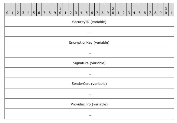
**SecurityID (variable):** Contains the sender <u>SID</u> or the sending queue manager <u>GUID</u>. This field MUST be set to the queue manager **GUID** when the packet is sent and signed by the queue manager.
