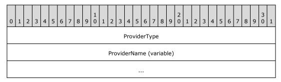
**ProviderType (4 bytes):** A 32-bit unsigned integer that indicates the type of the alternative provider used to produce the signature.
