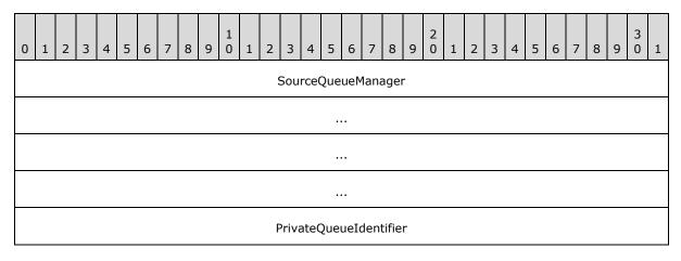
**SourceQueueManager (16 bytes):** A **GUID**, as specified in [MS-DTYP] section 2.3.4, that MUST specify the queue manager that hosts the private queue. The start of this field is rounded up to the next 4-byte boundary.
