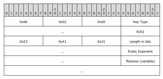
**Key Type (4 bytes):** This MUST be set to 0x00002400 for RSA signing keys and 0x0000A400 for RSA encryption keys.
