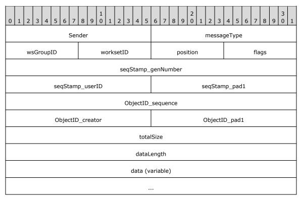
**Sender (2 bytes):** The local identifier of the user, which is obtained from the Multipoint Communication Service (MCS) [T122] layer. For more information about the MCS user ID, see [T122] section 3 (Definitions) in the ITU-T Recommendation.
