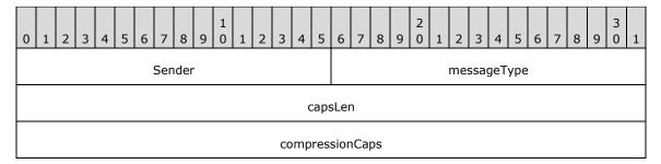
**Sender (2 bytes):** The local identifier of the user, which is obtained from the Multipoint Communication Service (MCS) [T122] layer. For more information about the MCS user ID, see [T122] section 3 (Definitions) in the ITU-T Recommendation.
