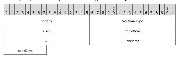
**length (2 bytes):** The length, in bytes, of the packet including the 2 bytes required for this length value.
