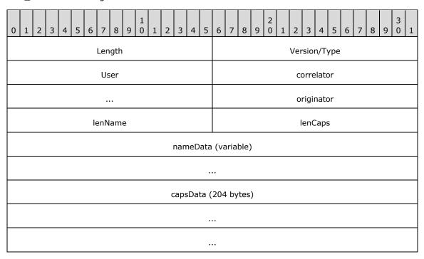
**Length (2 bytes):** The length, in bytes, of the packet including the 2 bytes required for this length value.
