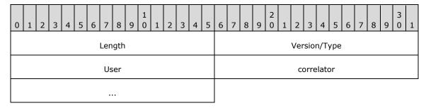
**Length (2 bytes):** The length, in bytes, of the packet including the 2 bytes required for this length value.
