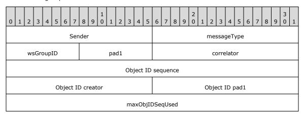
**Sender (2 bytes):** The local identifier of the user, which is obtained from the Multipoint Communication Service (MCS) [T122] layer. For more information about the MCS user ID, see [T122] section 3 (Definitions) in the ITU-T Recommendation.
