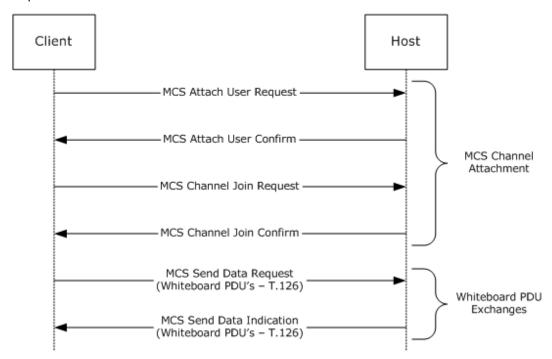
Figure 11: Typical sequencing during a whiteboard exchange
