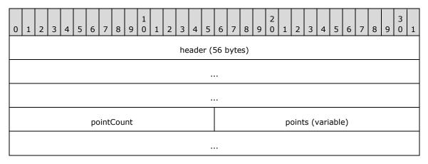
**header (56 bytes):** The basic information about the drawing. A <u>WB\_GRAPHIC</u> structure.
