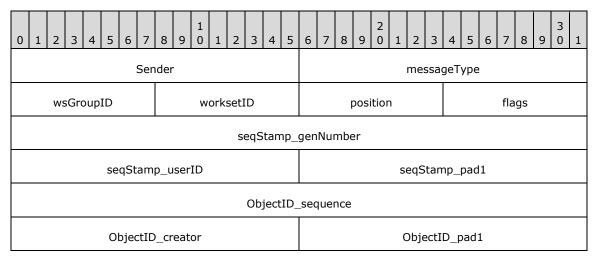
**Sender (2 bytes):** The local identifier of the user, which is obtained from the Multipoint Communication Service (MCS) [T122] layer. For more information about the MCS user ID, see [T122] section 3 (Definitions) in the ITU-T Recommendation.
