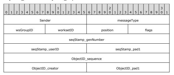
**Sender (2 bytes):** The local identifier of the user, which is obtained from the Multipoint Communication Service (MCS) [T122] layer. For more information about the MCS user ID, see [T122] section 3 (Definitions) in the ITU-T Recommendation.
