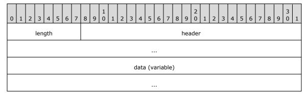
length (1 byte): The length of the header, including this field. MUST be set to 0x08.
