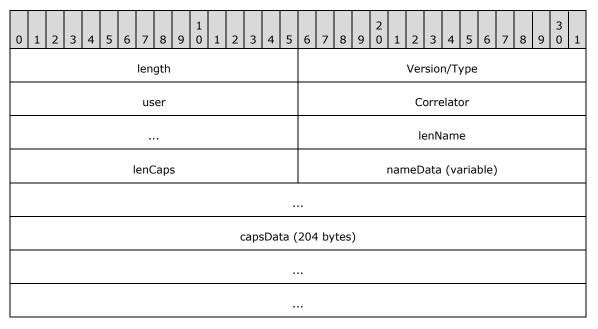
**length (2 bytes):** The length, in bytes, of the packet including the 2 bytes required for this length value.
