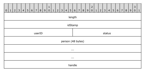
length (4 bytes): The byte length of this data packet, exclusive of the byte length of this field.
