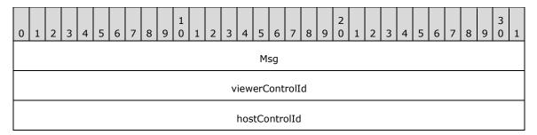
**Msg (4 bytes):** MUST contain either the value 0x00008003 for a pause or the value 0x00008004 for an unpause.
