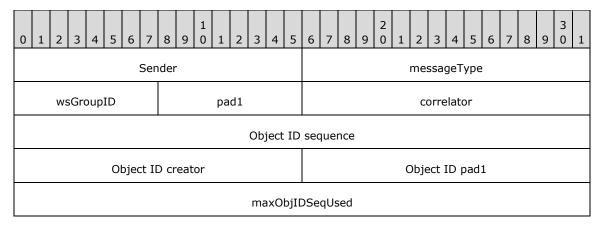
**Sender (2 bytes):** The local identifier of the user, which is obtained from the Multipoint Communication Service (MCS) [T122] layer. For more information about the MCS user ID, see [T122] section 3 (Definitions) in the ITU-T Recommendation.
