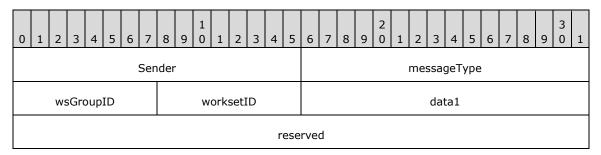
**Sender (2 bytes):** The local identifier of the user, which is obtained from the Multipoint Communication Service (MCS) [T122] layer. For more information about the MCS user ID, see [T122] section 3 (Definitions) in the ITU-T Recommendation.
