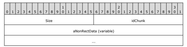
Size (2 bytes): The size, in bytes, of this structure.
