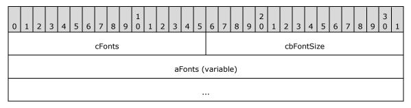
**cFonts (2 bytes):** The number of <u>NETWORKFONT</u> structures in **aFonts**.
