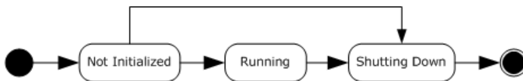
Figure 5: State machine diagram for the server
