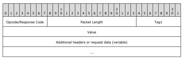
**Opcode/Response Code (1 byte):** This value can be used as an opcode (in the request message) or as a response code (in the response message), and it defines the IrOBEX operation associated with this packet, as defined in <a href="IROBEX">[IROBEX]</a> section 3.3. If this message is a response message, as defined in <a href="IROBEX">[IROBEX]</a> section 3.2, the response code value MUST be taken from <a href="IROBEX">[IROBEX]</a> section 3.2.1.
