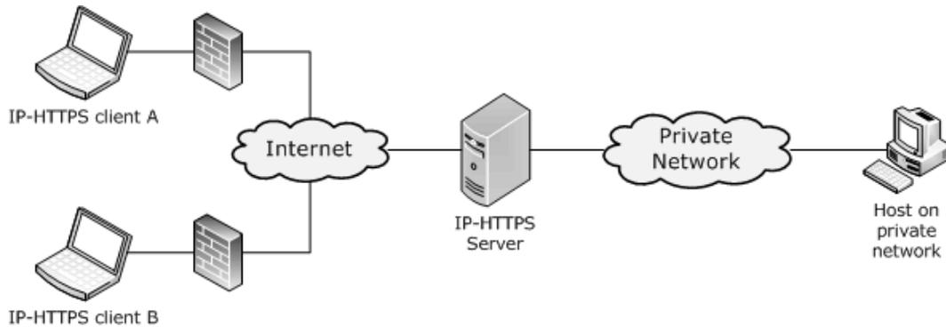
**Figure 5: IP-HTTPS clients connected to an IP-HTTPS server**
