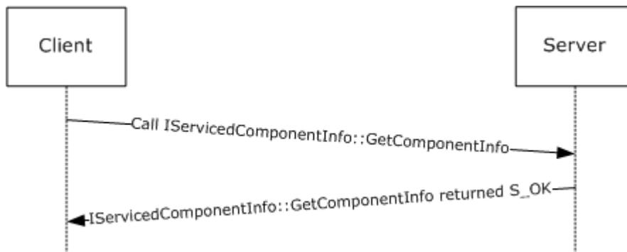
**Figure 4: Call sequence for determining server object identity**
