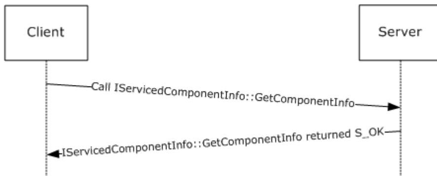
Figure 4: Call sequence for determining server object identity
