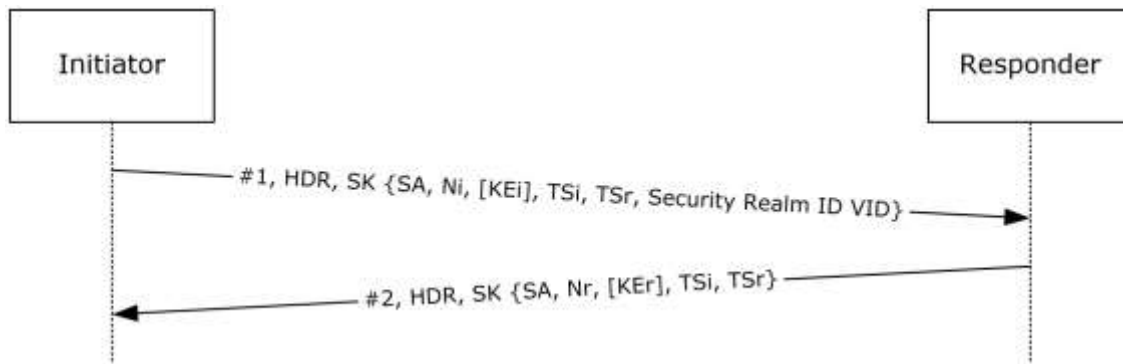
Figure 16: Sending Security Realm ID Vendor ID in IKE_SA_INIT and IKE_SA_AUTH messages
