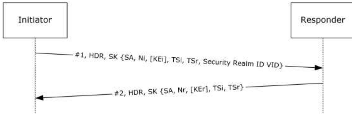
Figure 17: Sending Security Realm ID Vendor ID payload in CREATE_CHILD_SA messages
