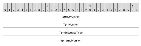
**StructVersion (4 bytes):** Structure version is set to 1.
