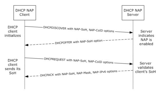
Figure 3: DHCP new lease acquisition process
