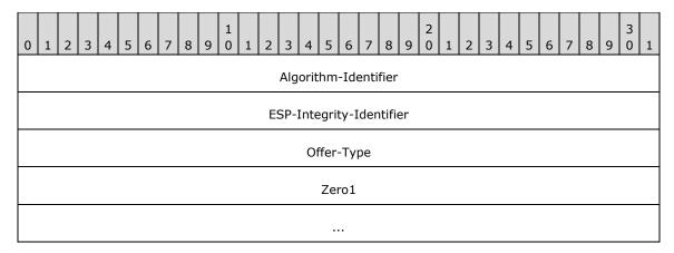
Algorithm-Identifier (4 bytes): The IPsec framing algorithm identifier; either AH or ESP.
