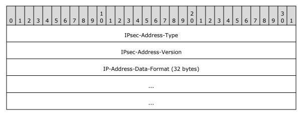
**IPsec-Address-Type (4 bytes):** Specifies the type of address that the IPsec filter specifies. This includes special filter types that have a predefined meaning and are interpreted based on the IP configuration of the host machine. This MUST be one of the following values and MUST be an unsigned integer.
