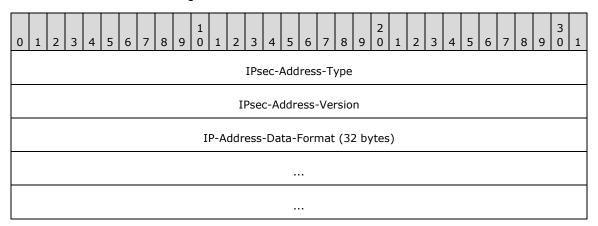
**IPsec-Address-Type (4 bytes):** Specifies the type of address that the IPsec filter specifies. This includes special filter types that have a predefined meaning and are interpreted based on the IP configuration of the host machine. This MUST be one of the following values and MUST be an unsigned integer.
