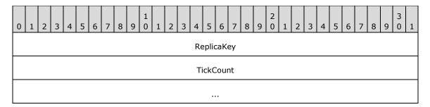
**ReplicaKey (4 bytes):** The index into the REPLICA\_KEY\_MAP to define the REPLICA\_GID entry for the replica described by this element.
