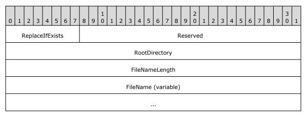
**ReplaceIfExists (1 byte):** A <u>Boolean (section 2.1.8)</u> value. Set to TRUE to indicate that if the link already exists, it SHOULD be replaced with the new link. Set to FALSE to indicate that the link creation operation MUST fail if the link already exists.
