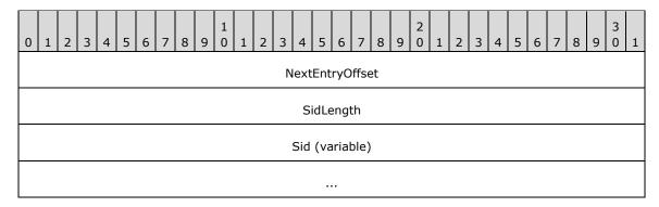
**NextEntryOffset (4 bytes):** A 32-bit unsigned integer that contains the byte offset from the beginning of this entry, at which the next FILE\_GET\_QUOTA\_INFORMATION entry is located, if multiple entries are present in a buffer. This member MUST be zero if no other entries follow this one. An implementation MUST use this value to determine the location of the next entry (if multiple entries are present in a buffer).
