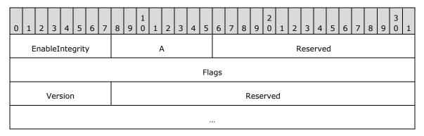
**EnableIntegrity (1 byte):** This field MUST be one of the following values:
