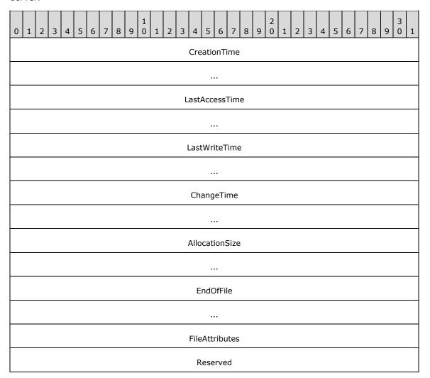
**CreationTime (8 bytes):** The time when the file was created; see section 2.1.1. The value of this field MUST be greater than or equal to 0.
