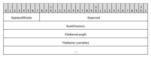
**ReplaceIfExists (1 byte):** A <u>Boolean (section 2.1.8)</u> value. Set to TRUE to indicate that if a file with the given name already exists, it SHOULD be replaced with the given file. Set to FALSE to indicate that the rename operation MUST fail if a file with the given name already exists.
