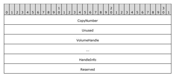
**CopyNumber (4 bytes)**: A 32-bit unsigned integer that identifies, when reading from a file which resides on redundant media, which copy to read.
