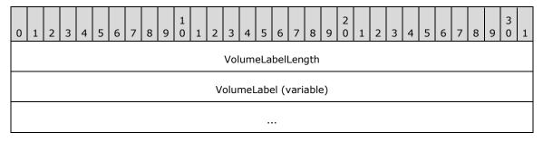
**VolumeLabelLength (4 bytes):** A 32-bit unsigned integer that contains the length, in bytes, including the trailing null, if present, of the name for the volume.<a href="mailto:<148"><148</a>>
