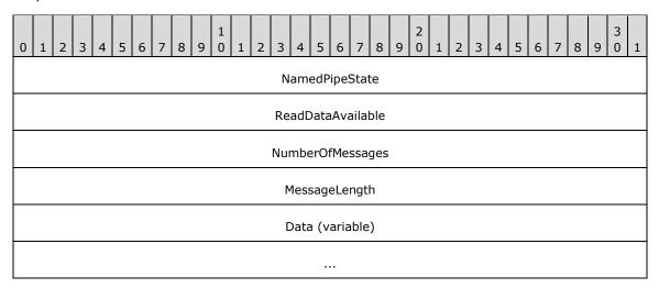
**NamedPipeState (4 bytes):** A 32-bit unsigned integer referring to the current state of the pipe. The allowed values are shown in the following table.
