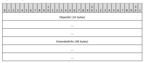
**ObjectId (16 bytes):** A 16-byte **GUID** that identifies the file system **volume** on the disk. This value is not required to be unique on the system.
