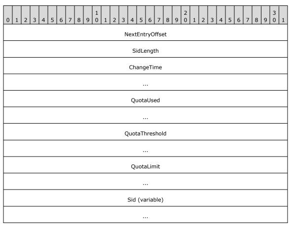
**NextEntryOffset (4 bytes):** A 32-bit unsigned integer that contains the byte offset from the beginning of this entry, at which the next FILE\_QUOTA\_INFORMATION entry is located, if multiple entries are present in a buffer. This member MUST be zero if no other entries follow this one. An
