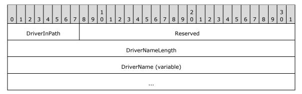
**DriverInPath (1 byte):** A <u>Boolean (section 2.1.8)</u> value. Set to TRUE if the driver is in the I/O path for the file system volume; set to FALSE otherwise.
