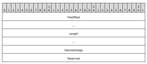
**FileOffset (8 bytes):** A 64-bit signed integer that contains the file offset, in bytes, of the start of a range of bytes in a file.
