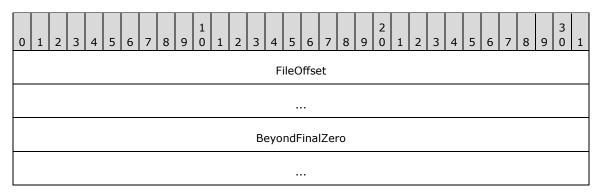
**FileOffset (8 bytes):** A 64-bit signed integer that contains the file offset of the start of the range to set to zeros, in bytes. The value of this field MUST be greater than or equal to 0.
