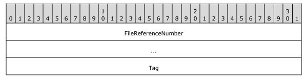
FileReferenceNumber (8 bytes): The 64-bit file ID, as specified in section 2.1.9, for the file.
