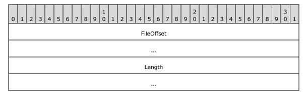
**FileOffset (8 bytes):** A 64-bit signed integer that contains the file offset, in bytes, of the start of a range of bytes in a file. The value of this field MUST be greater than or equal to 0.
