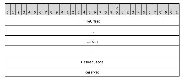
FileOffset (8 bytes): A 64-bit signed integer that contains the file offset, in bytes, of the region.
