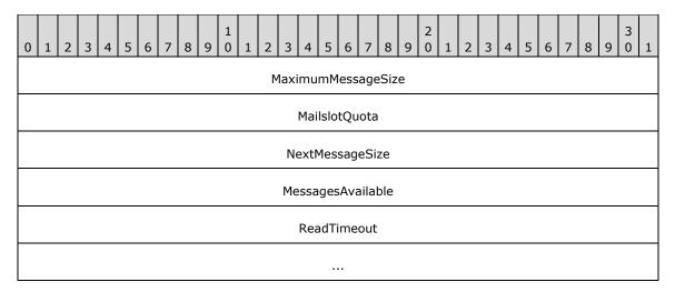
**MaximumMessageSize (4 bytes):** A 32-bit unsigned integer that contains the maximum size of a single message that can be written to the mailslot, in bytes. To specify that the message can be of any size, set this value to zero.
