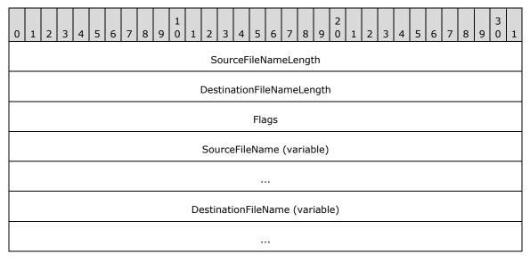
**SourceFileNameLength (4 bytes):** A 32-bit unsigned integer that contains the size, in bytes, of the **SourceFileName** element, including a terminating-Unicode null character.
