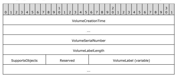
**VolumeCreationTime (8 bytes):** The time when the volume was created; see section 2.1.1. The value of this field MUST be greater than or equal to 0.
