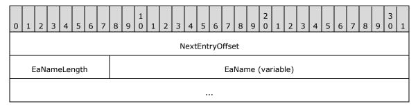
**NextEntryOffset (4 bytes):** A 32-bit unsigned integer that contains the byte offset from the beginning of this entry, at which the next **FILE\_GET\_EA\_INFORMATION** entry is located, if multiple entries are present in a buffer. This member MUST be zero if no other entries follow this one. An implementation MUST use this value to determine the location of the next entry (if multiple entries are present in a buffer).
