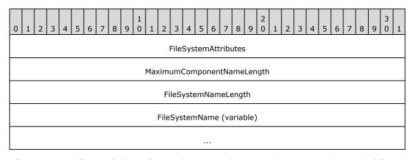
FileSystemAttributes (4 bytes): A 32-bit unsigned integer that contains a bitmask of flags that specify attributes of the specified file system as a combination of the following flags. The value of this field MUST be a bitwise OR of zero or more of the following with the exception that FILE\_FILE\_COMPRESSION and FILE\_VOLUME\_IS\_COMPRESSED cannot both be set. Any flag values not explicitly mentioned here can be set to any value, and MUST be ignored.<a href="mailto:<138"><138</a>>
