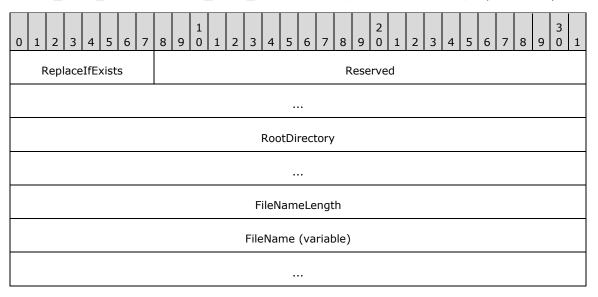
**ReplaceIfExists (1 byte):** A <u>Boolean (section 2.1.8)</u> value. Set to TRUE to indicate that if the link already exists, it SHOULD be replaced with the new link. Set to FALSE to indicate that the link creation operation MUST fail if the link already exists.
