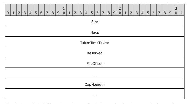
Size (4 bytes): A 32-bit unsigned integer that indicates the size, in bytes, of this data element.
