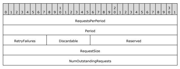
**RequestsPerPeriod (4 bytes):** A 32-bit unsigned integer indicating the number of I/O requests that complete per period of time, as specified in the **Period** field. When setting bandwidth reservation, a value of 0 indicates to the file system that it MUST free any existing reserved bandwidth.
