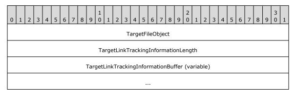
**TargetFileObject (4 bytes):** The **Fid** of the file from which to obtain link tracking information. For Fid type, see [MS-SMB] section 2.2.7.2.1.
