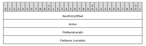
**NextEntryOffset (4 bytes):** The offset, in bytes, from the beginning of this structure to the subsequent **FILE\_NOTIFY\_INFORMATION** structure. If there are no subsequent structures, the **NextEntryOffset** field MUST be 0. **NextEntryOffset** MUST always be an integral multiple of 4. The **FileName** array MUST be padded to the next 4-byte boundary counted from the beginning of the structure.
