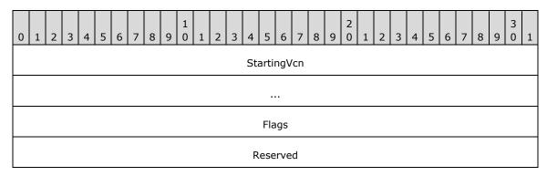
**StartingVcn (8 bytes):** A signed integer representing the starting VCN for which to perform the request on.
