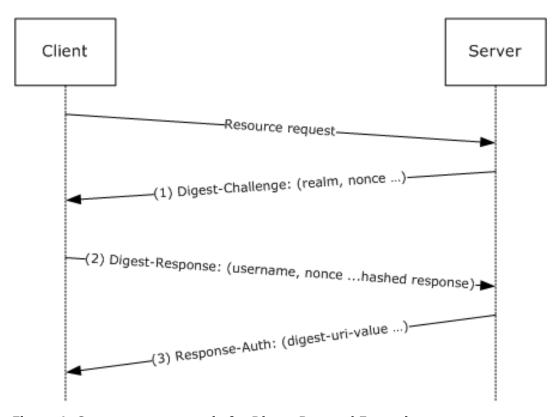
Figure 1: Common use scenario for Digest Protocol Extensions
