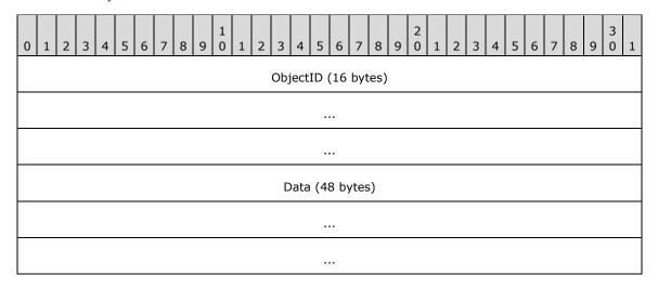
**ObjectID (16 bytes):** A 16-byte GUID, as specified in [MS-DTYP] section 2.3.4.2, assigned by the server on which the file is stored, that uniquely identifies the file or directory within the volume in which it is stored.
