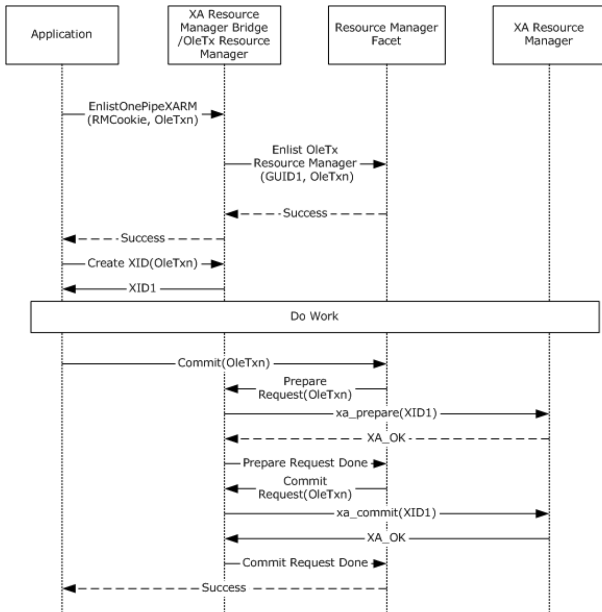
Figure 11: One-pipe XA Resource Manager transaction enlistment and completion
