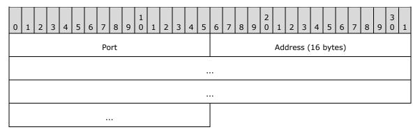
**Port (2 bytes):** IPv6 port. This MUST be greater than or equal to 1024.
