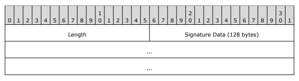
**Length (2 bytes):** The number of bytes, in **little-endian** byte order, of the structure. MUST be set to 130 bytes.
