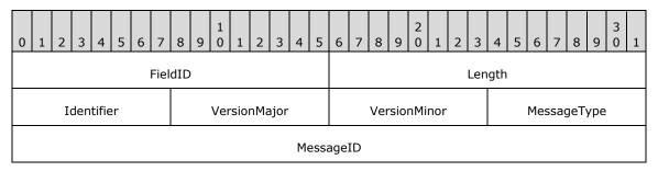
FieldID (2 bytes): The type of message. It MUST be set to 0x0010 (DRT\_HEADER).
