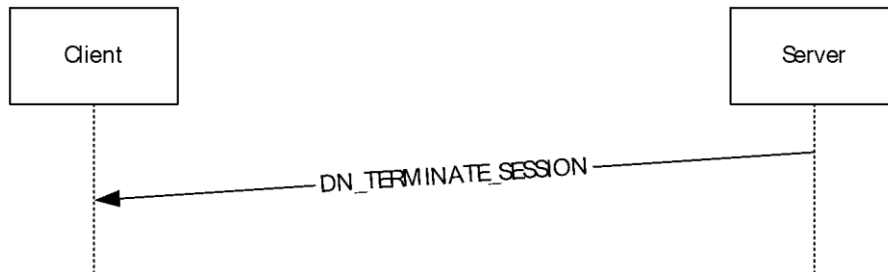
Figure 12: Client/server disconnect sequence
